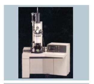
Figure 13 Philips CM 10 electron microscope (1990 – present).
