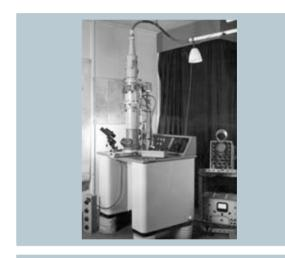
**Figure 2** Metropolitan Vickers EM 3A electron microscope (1960).
