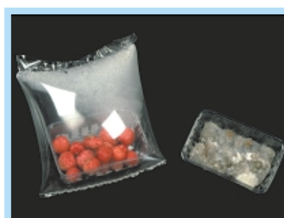
Figure 6 Strawberry packaged in 80% O 2 : 20% N 2 after 60 days and a control open container.
