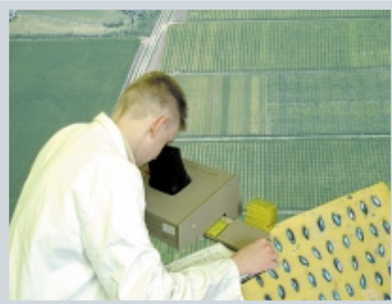
Figure 3 Assessing evenness of barley cell wall modification following malting using a fluorescent dye.
