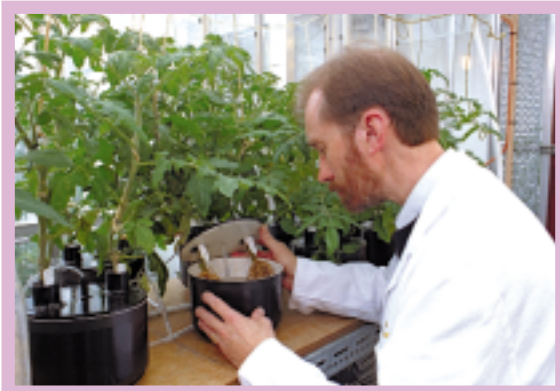
Figure 3 A hydroponic system for growing infected tomato to produce the millions of nematodes needed to collect their secretions.
