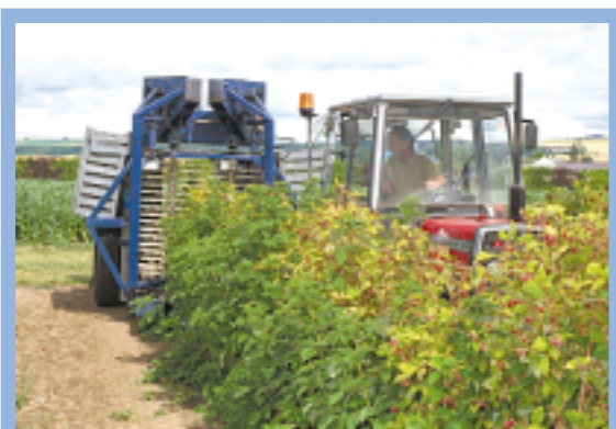
Figure 5 Promising raspberry selections are evaluated for machine harvesting using a Korvan raspberry harvester.
