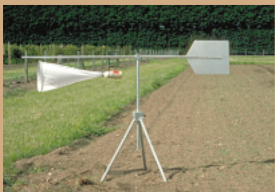
Figure 5 Swinging net trap to catch live aphids.
