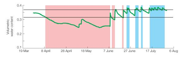
Figure 1 Variation in the volumetric water content of soil over time at SCRI showing periods when roots were likely to be limited by mechanical impedance (pink) and shortage of oxygen (blue).
